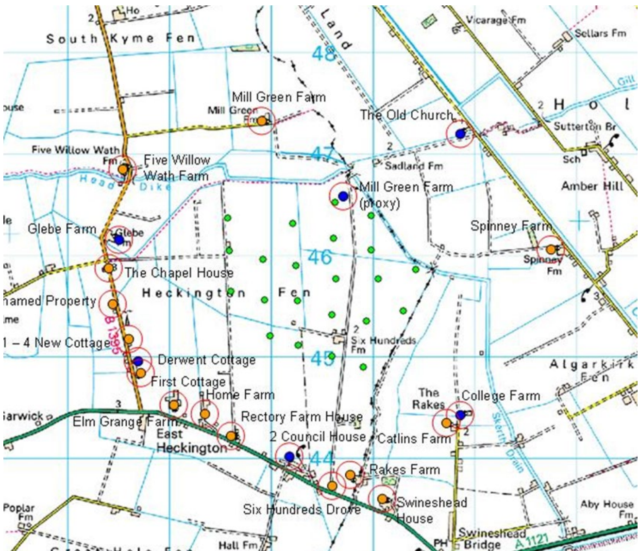
Figure 12.1.1 – Historical March 2011 Background noise survey locations (blue) and noise sensitive receptor locations (orange) from the Heckington Fen Wind Park application.
